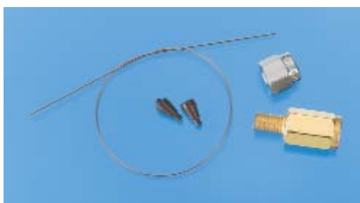
Figure 1 The EZ No-Vent™ connector incorporates a laser machined orifice for optimal flow through the fitting. Coupled with the 100µm ID transfer line, it minimizes the amount of oxygen entering the MS, which eliminates the need for purge gases.
